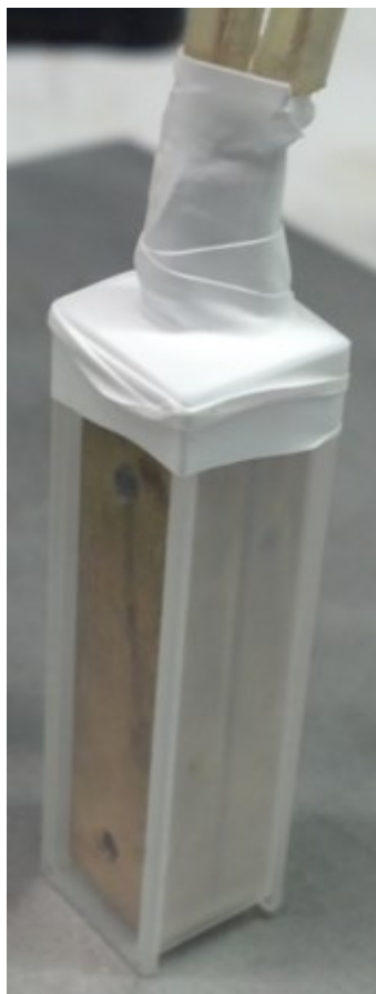
Figure 3.4: A picture of the capacitor submerged into the cuvette prior to placing into the oven.
