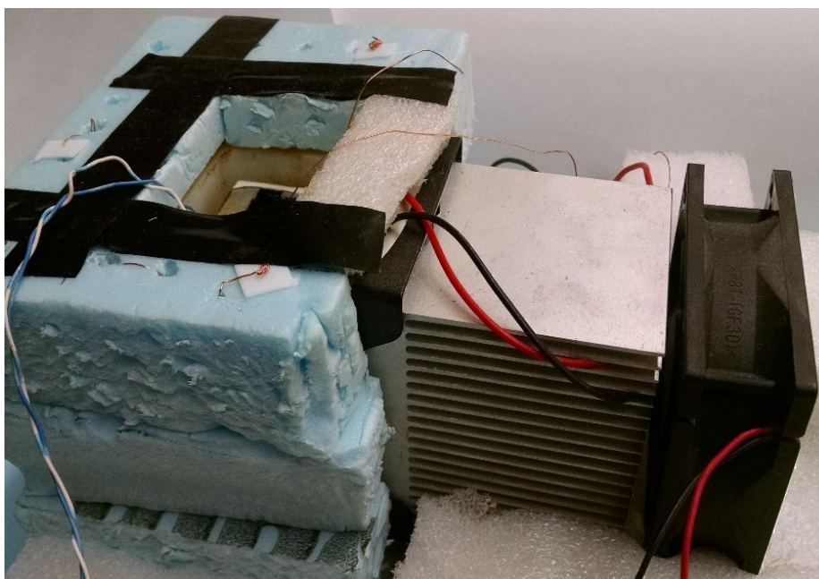
Figure 3.3: A photograph of the experimental setup and oven without the capacitor.
